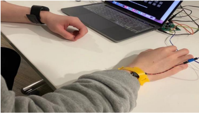
Figure 2: Setup of Experiment 1: Empatica E4 on the left wrist, vibrotactile actuator attached to wrist of right hand with a strap.
